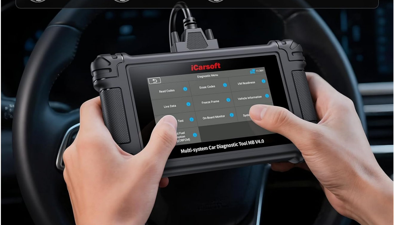
Figure 7: The iCarsoft MB V4.0 showing its comprehensive full OBD2 diagnostic functions.
