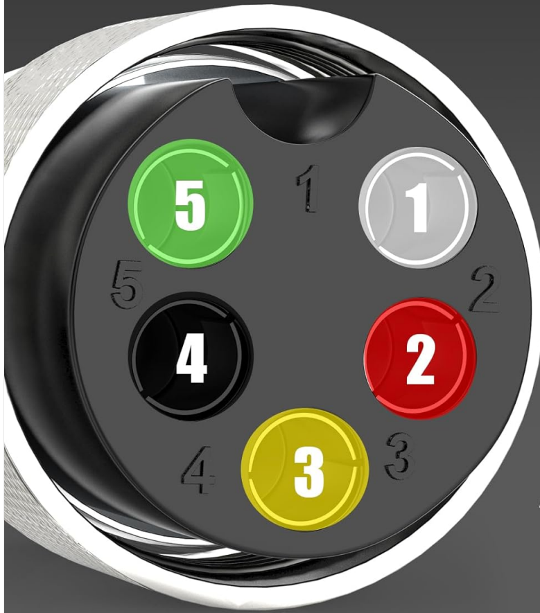
Image: A detailed view of the 5-pin plug for the foot pedal, indicating pins 3 & 5 for control switch and pins 1, 2 & 4 for amperage adjustment.
