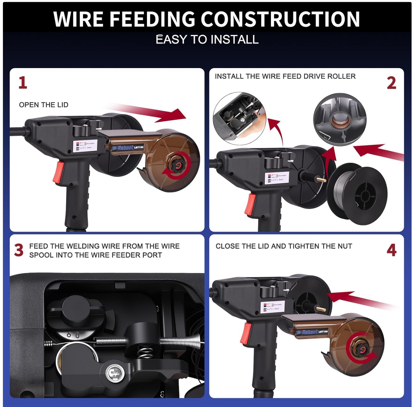
Image: A four-step visual guide for wire feeding construction. 1. Open the lid of the wire feeder. 2. Install the wire feed drive roller. 3. Feed the welding wire from the wire spool into the wire feeder port. 4. Close the lid and tighten the nut.
