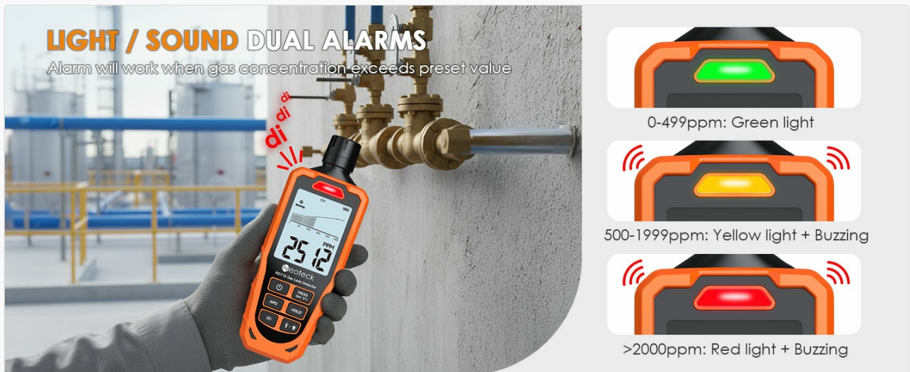
Image: Visual and audible alarm system with LED indicators.
