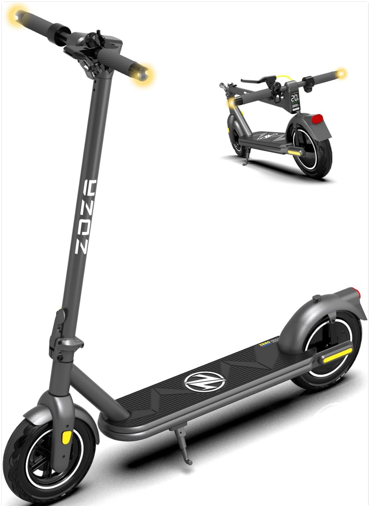
Image: Turn Signals and Taillight. This image shows the illuminated turn signals on the handlebar ends and the rear taillight, which also serves as a brake light.
