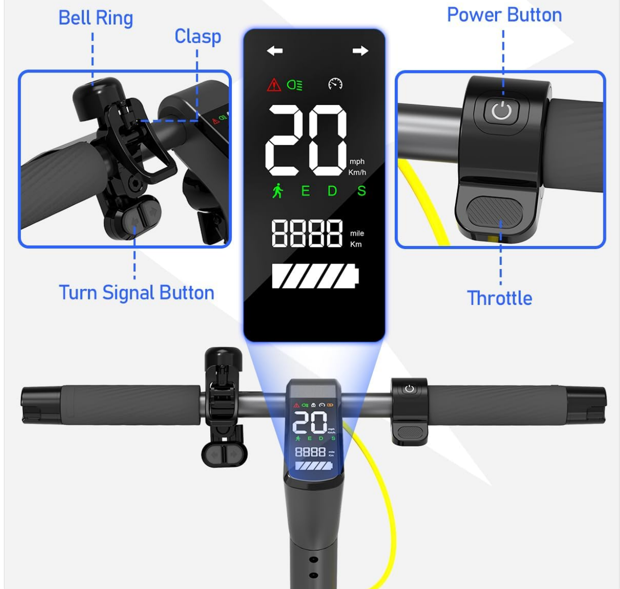
Image: All-in-one integrated Handlebars. This image highlights the various controls and the digital display on the scooter's handlebar, including the bell, turn signal buttons, power button, and throttle.
