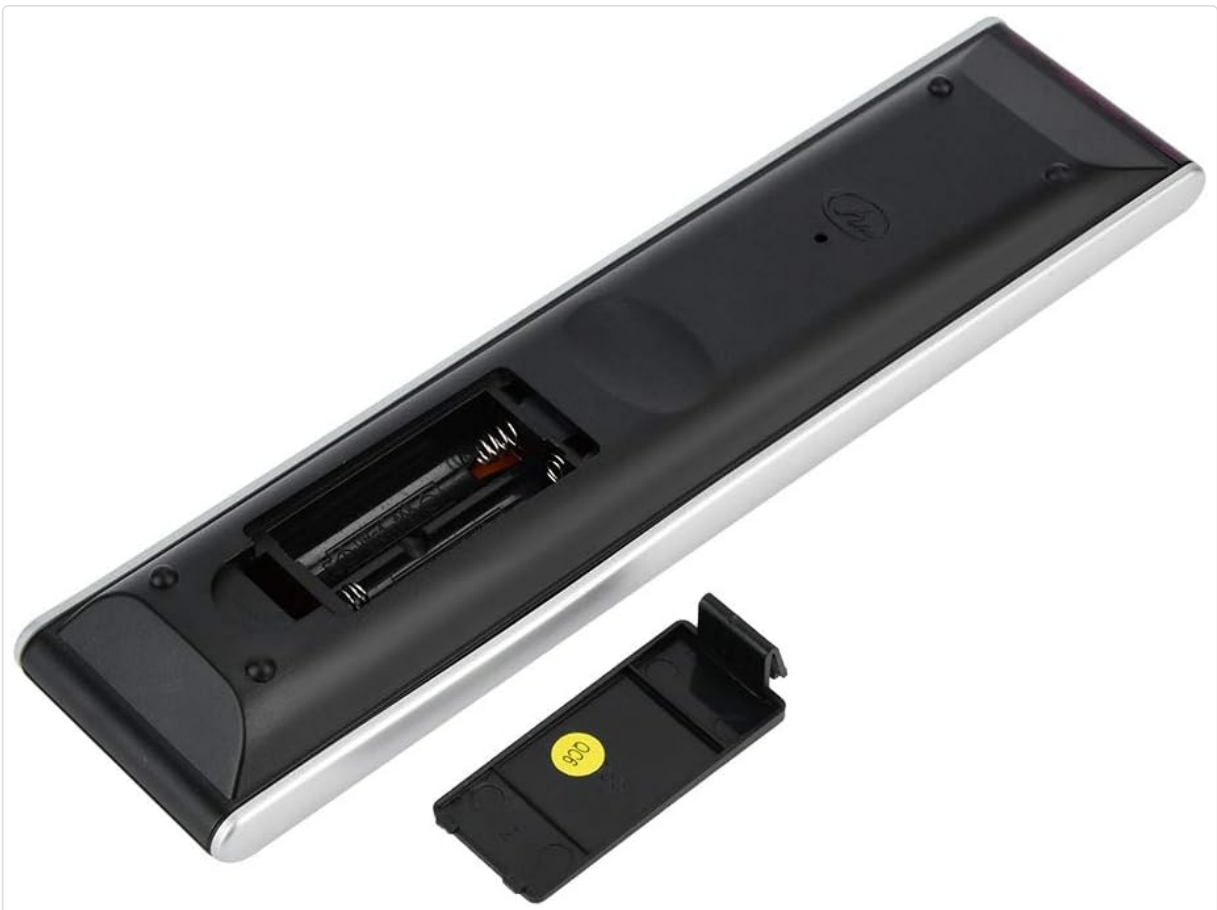
Image 3.1: The back of the Aumotop CT-90287A remote control with the battery compartment cover removed, showing the slots for two AAA batteries and the 'QC6' quality control sticker.
