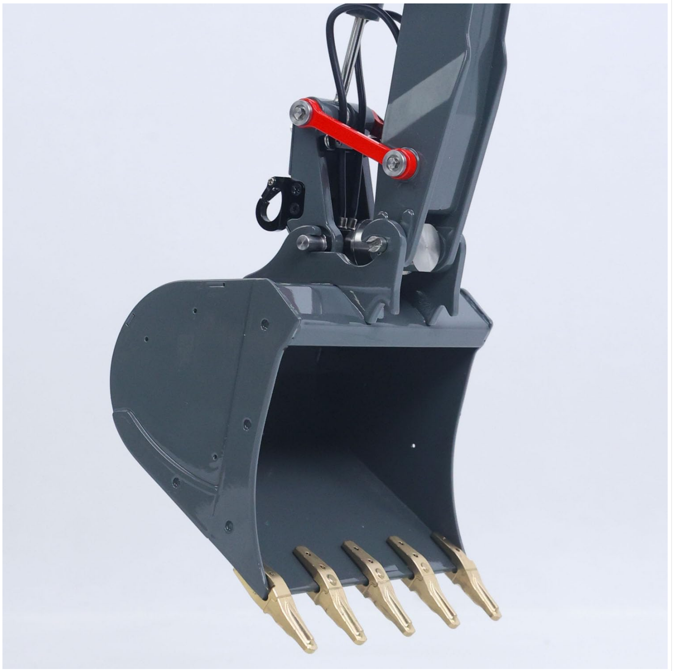
Figure 5: Close-up of the excavator bucket and its hydraulic connections.
