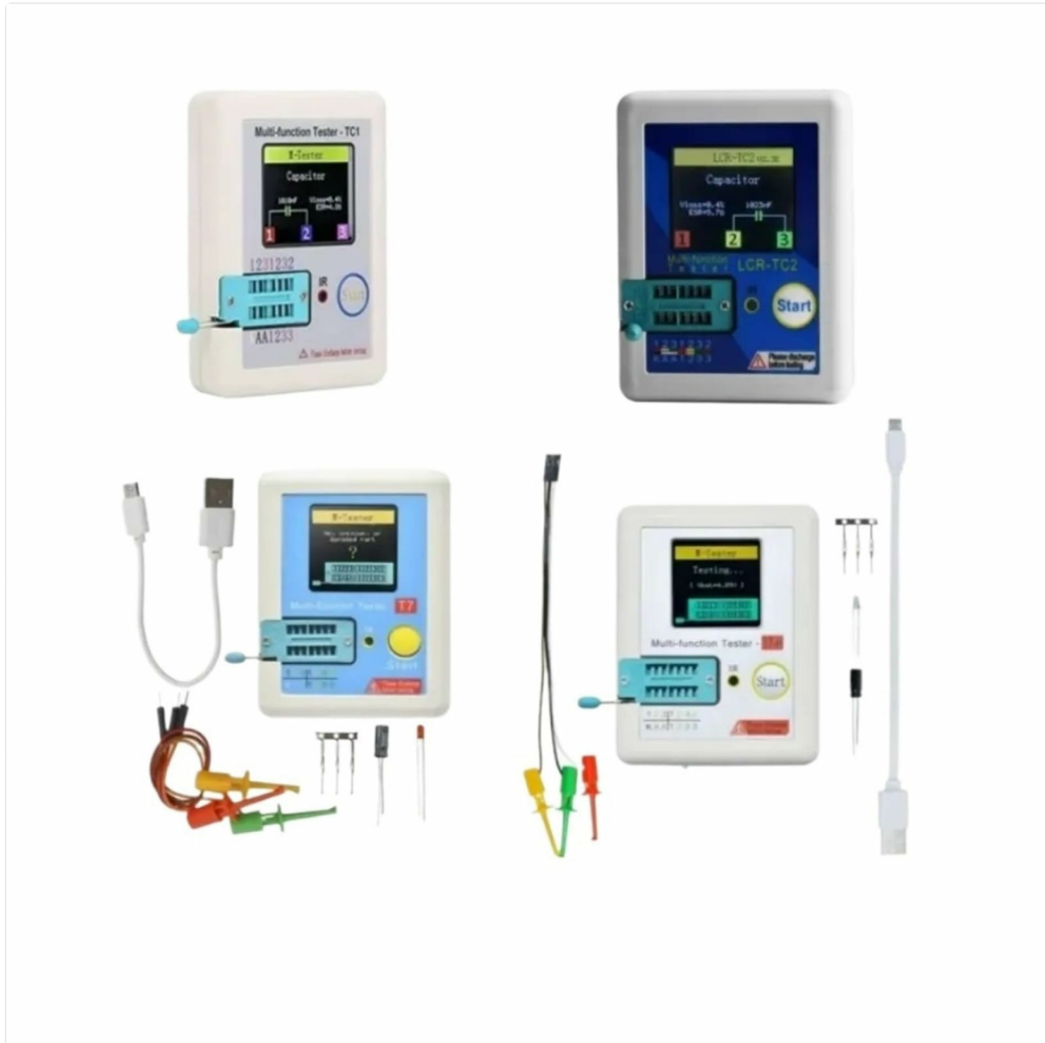
Image: A clear view of the LCR-TC2's front panel, highlighting the TFT color display, the 'Start' multi-function button, and the component test socket.
