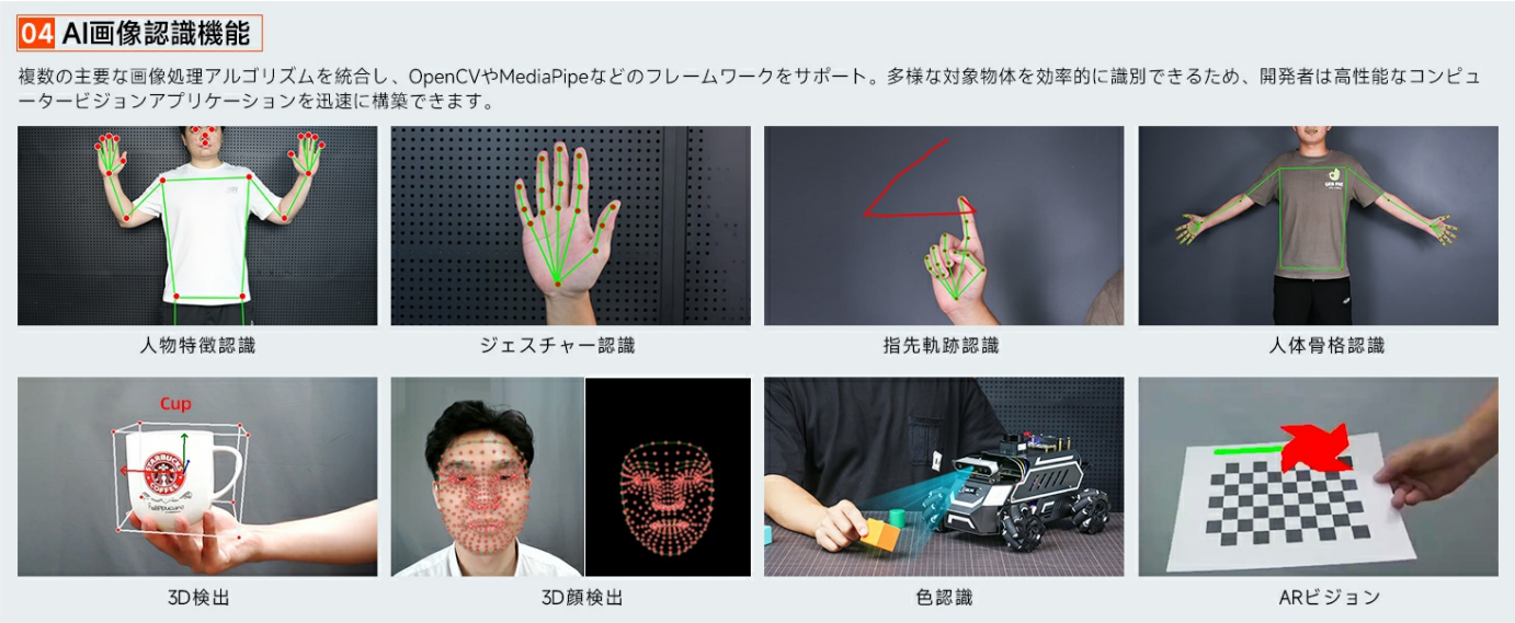
Image: Rosmaster M1 AI image recognition. This image showcases the robot's ability to perform various AI image recognition tasks, including human body recognition, gesture recognition, fingertip recognition, human skeleton recognition, 3D detection, 3D face detection, color recognition, and AR vision.
