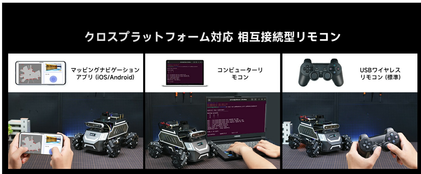
Image: Rosmaster M1 control methods. This image shows the robot being controlled via a smartphone app, a laptop, and a USB wireless gamepad.
