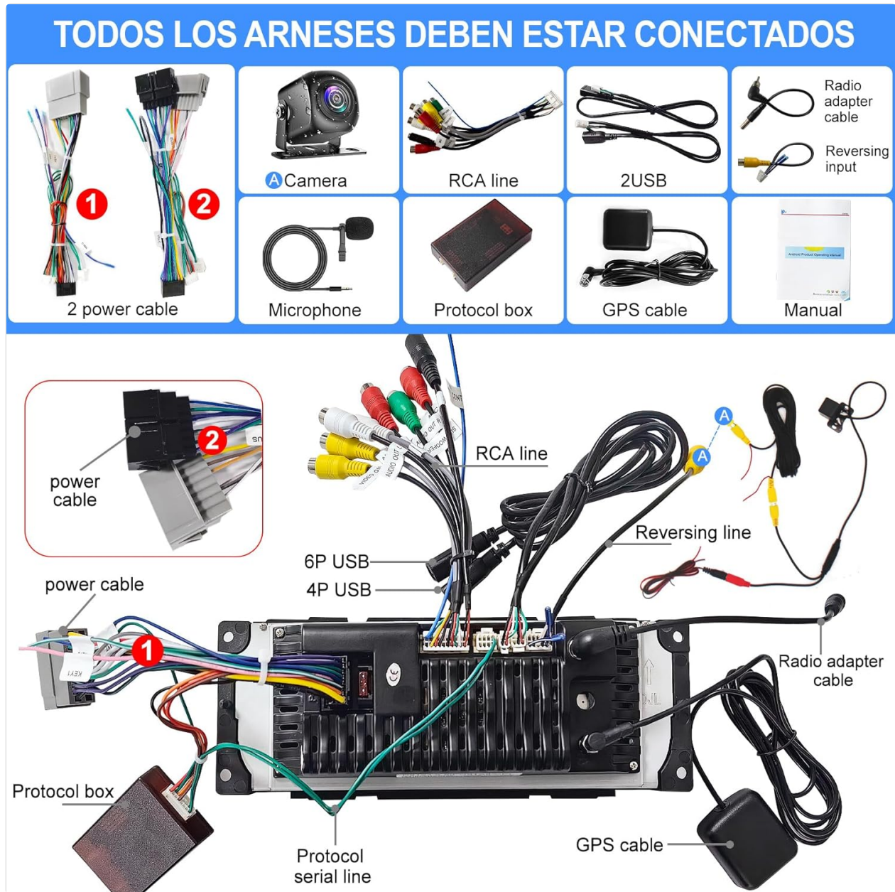
Image 4.1: Comprehensive wiring diagram showing connections for power, RCA, USB, microphone, GPS, and backup camera.
