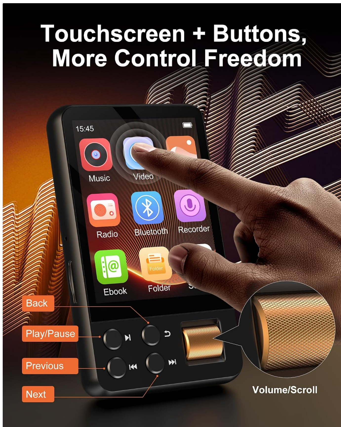
Image 4.1: A detailed diagram of the AGXOV D28 MP3 Player, highlighting its touchscreen interface and physical buttons for navigation
