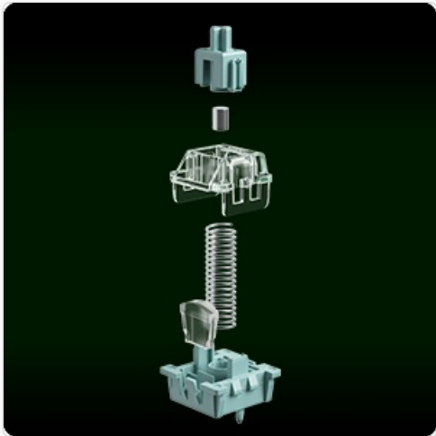
Image: Components of an AstroAim Magnetic Switch, illustrating its design for easy replacement.
