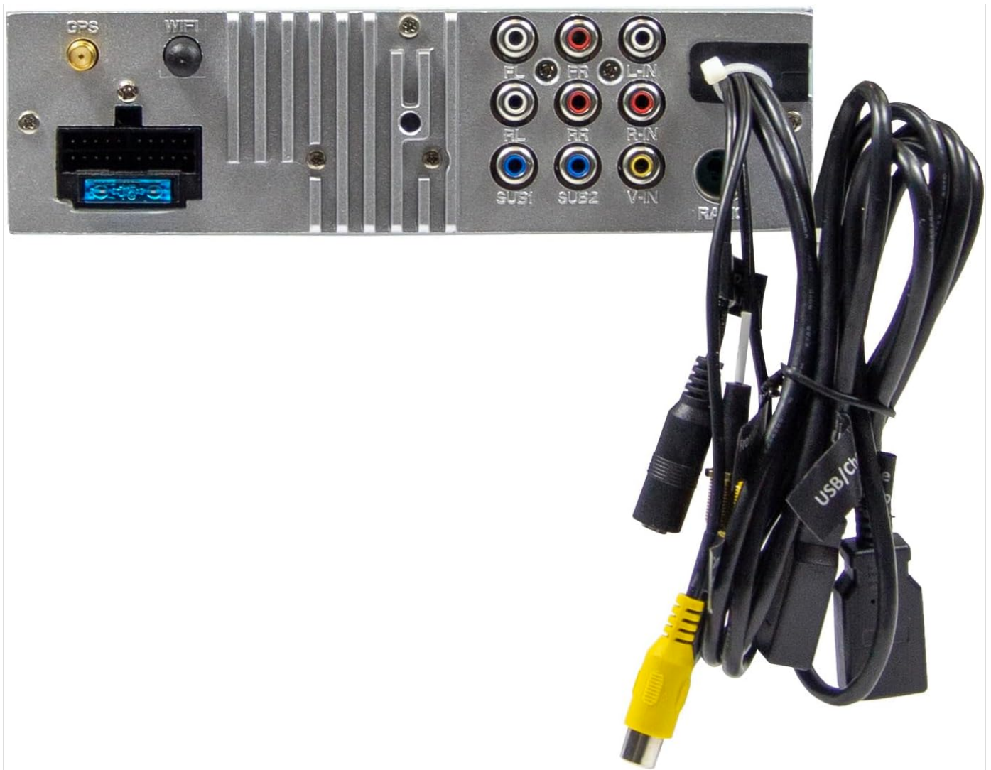
Image: Rear connections of the VMX1000DAB unit.
