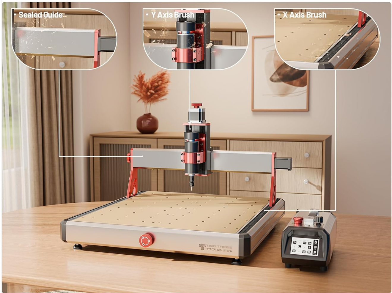
Figure 3.5.1: Details of the dustproof design, including sealed guides and axial brushes for enhanced durability and reduced maintenance.
