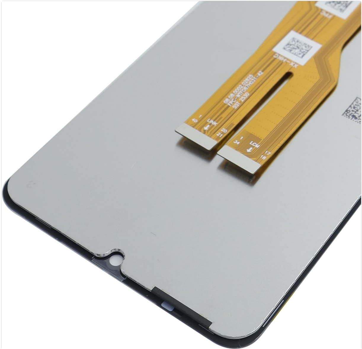
Image 3.1: Close-up of the display's flex cables, which connect to the motherboard for testing and installation.
