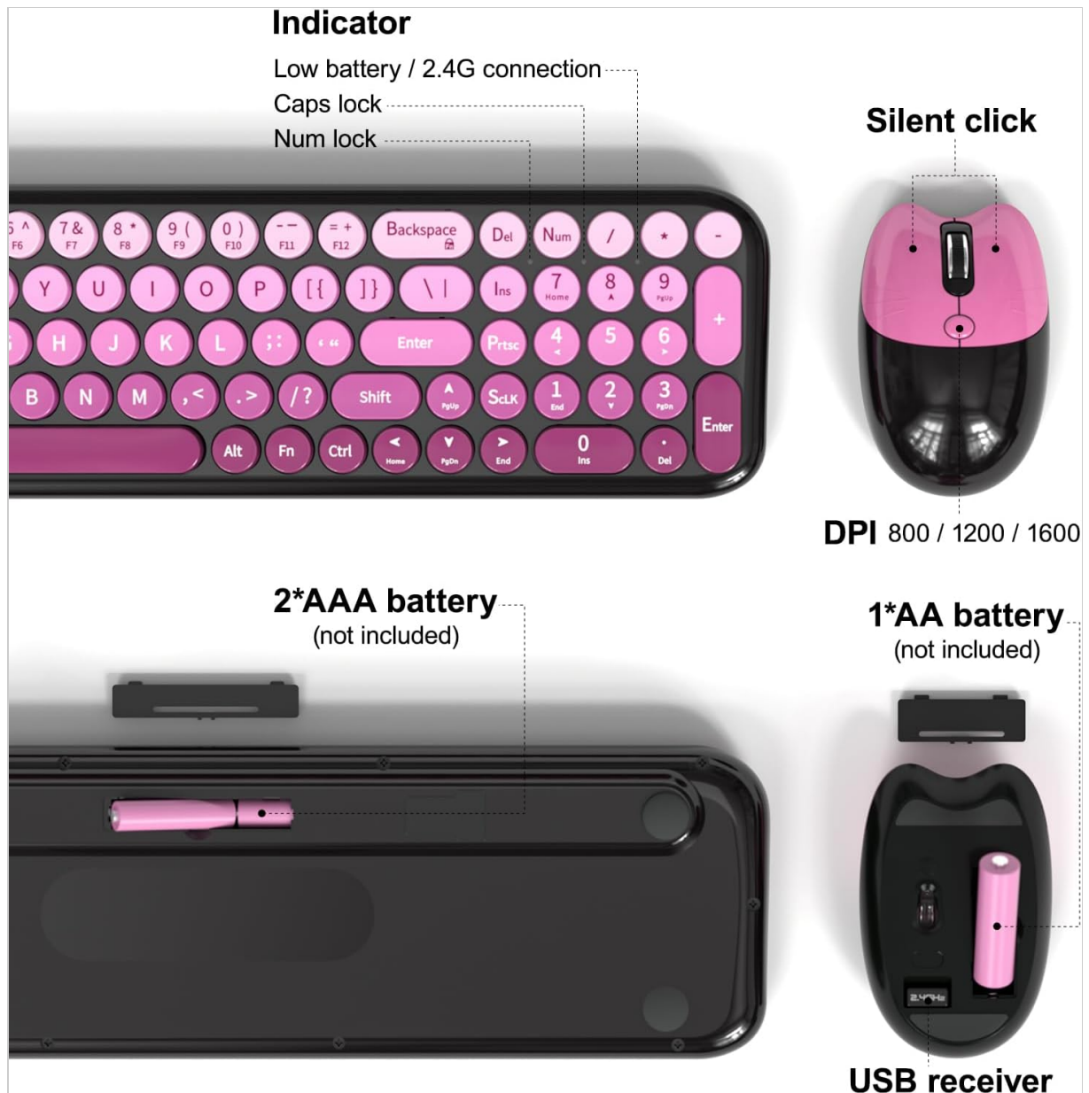
Image 2.1: Battery compartments for the keyboard (2xAAA) and mouse (1xAA).
