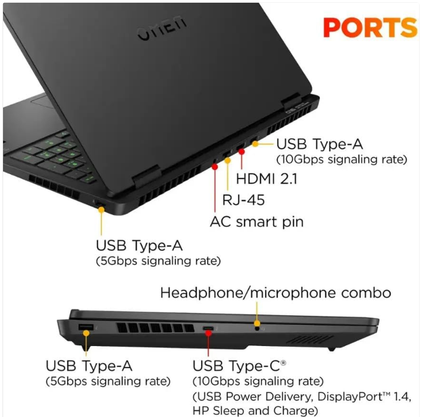
Image: Detailed diagram illustrating the port layout on the HP Omen 16-AN0075CL laptop.
