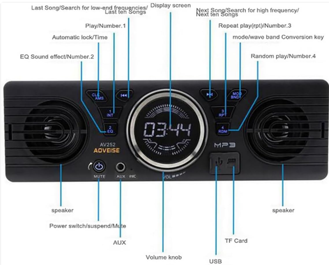
Image: Diagram illustrating the front panel controls of the AV252B unit, with labels for each button and port.
