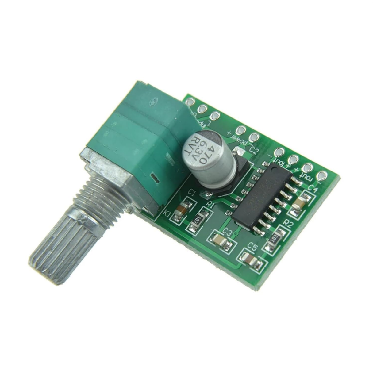
Figure 3.1: Top-down view of the PAM8403 amplifier board. This image shows the overall layout, including the volume control potentiometer on the left, the PAM8403 chip, and the clearly labeled connection pads for power input, audio input, and speaker outputs.
