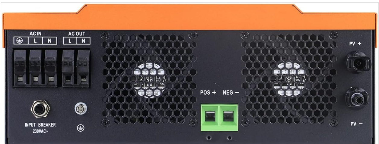
Image 3: Close-up of the inverter's rear panel showing AC input, AC output, PV input terminals (PV+ and PV-), and battery input terminals (POS+ and NEG-). Also visible are the input breaker and grounding screw.
