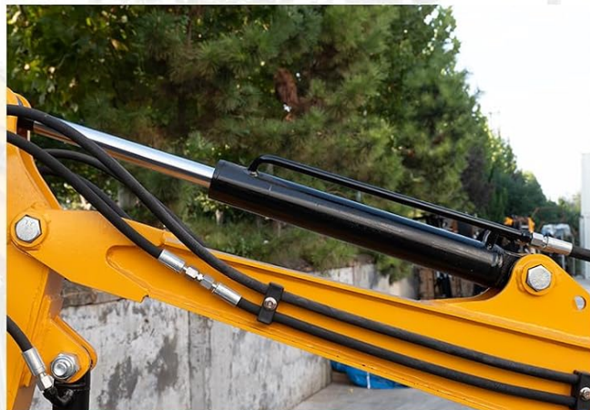
High pressure oil pipes
