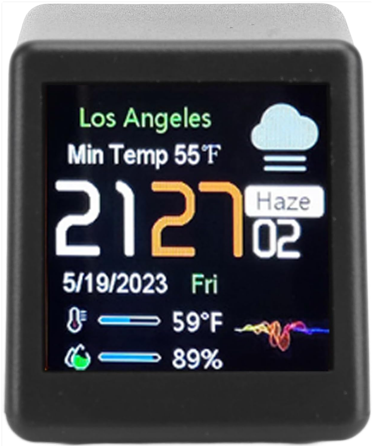
Image: A detailed close-up of the clock's LCD screen, clearly showing the city, minimum temperature, current time, date, weather condition (haze), current temperature, and humidity percentage.
