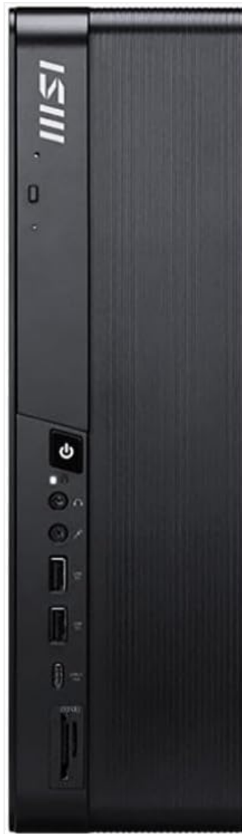
Image: Direct front view of the MSI PRO DP80 A14G desktop computer, highlighting the vertical textured panel with the MSI logo, power button, audio jacks, USB ports, and an SD card reader.
