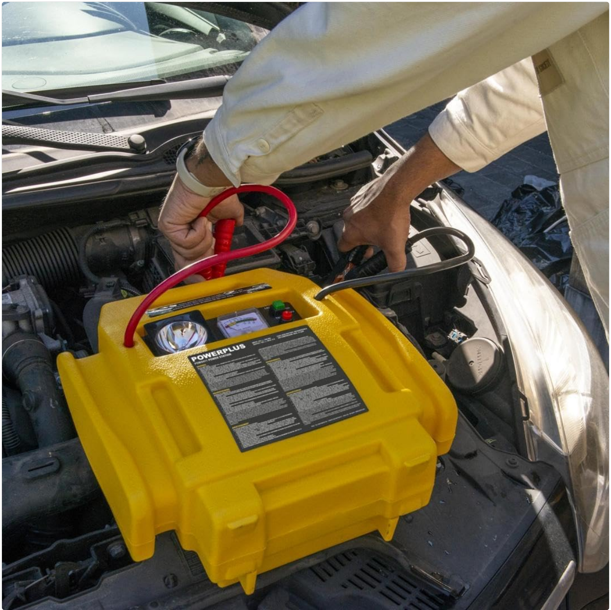
Figure 4: Connecting the jump starter clamps to a vehicle battery.
