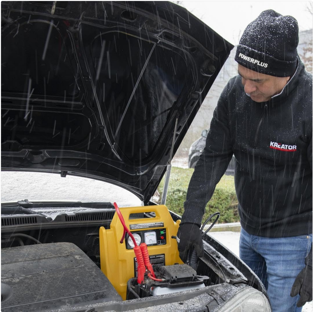
Figure 5: Using the Powerstation to jump start a car in cold weather.
