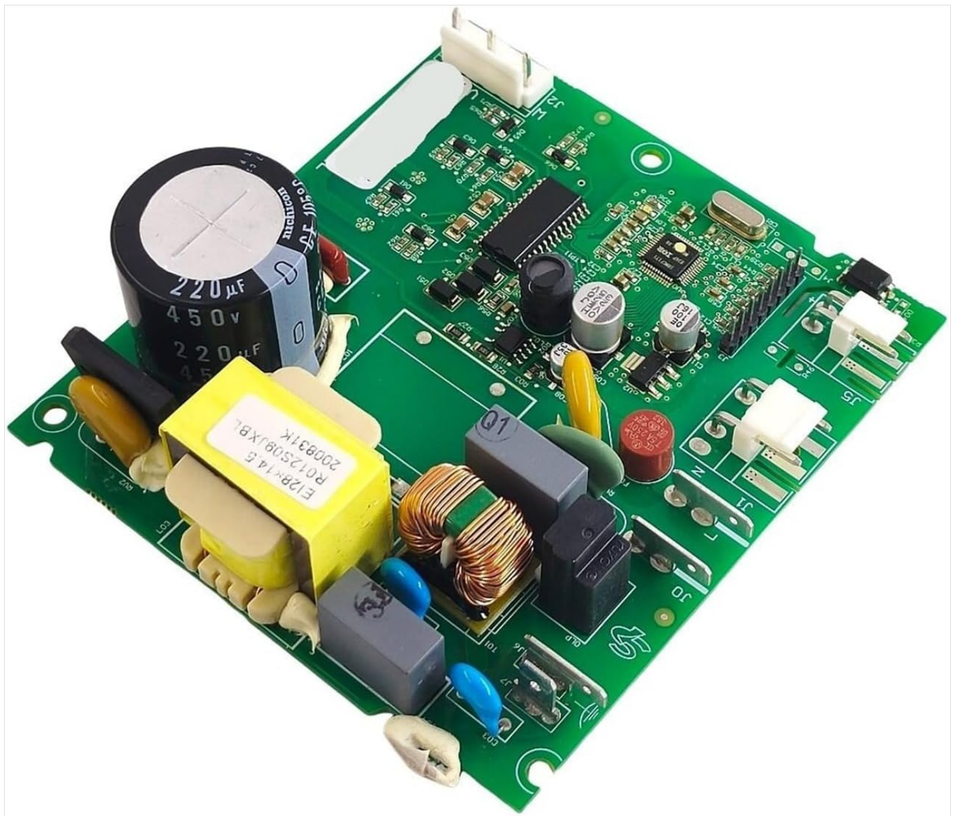
Figure 2: Angled perspective of the board, showing the main power components and connection points.
