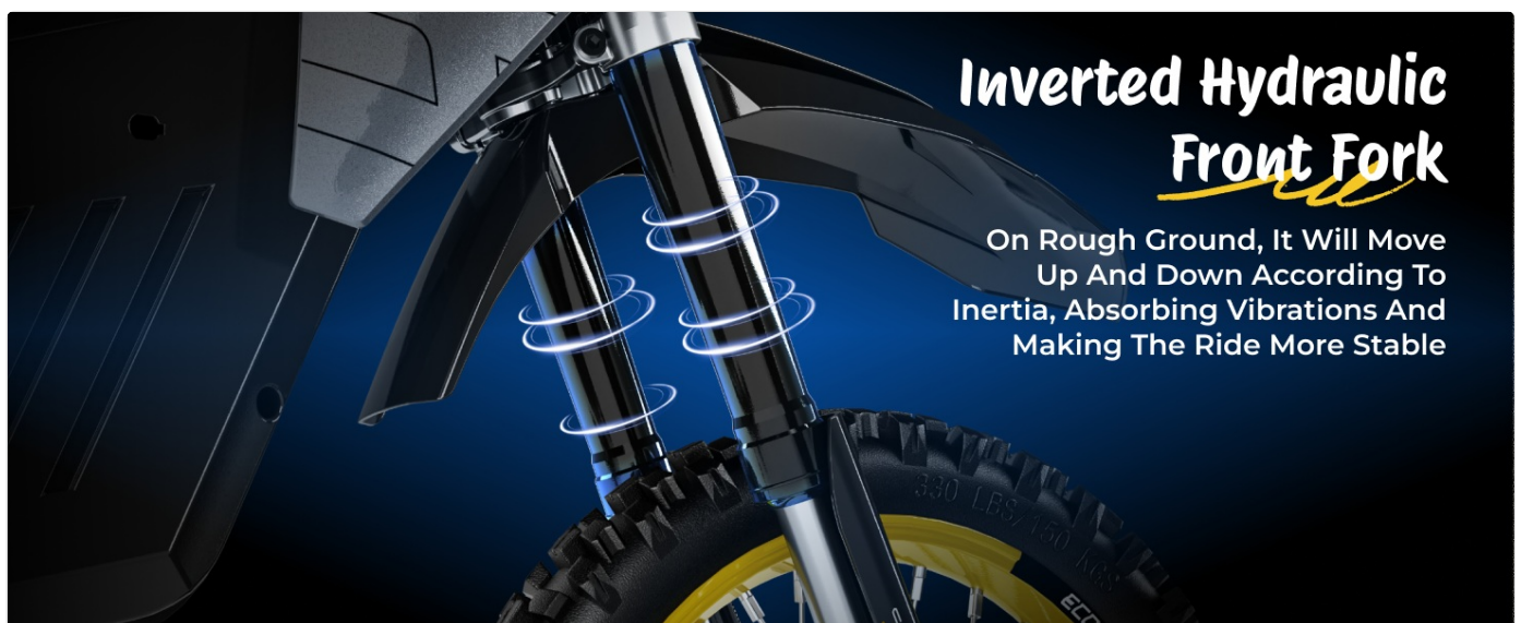
Image: Close-up view of the inverted hydraulic front fork, designed to absorb vibrations for a more stable ride.
