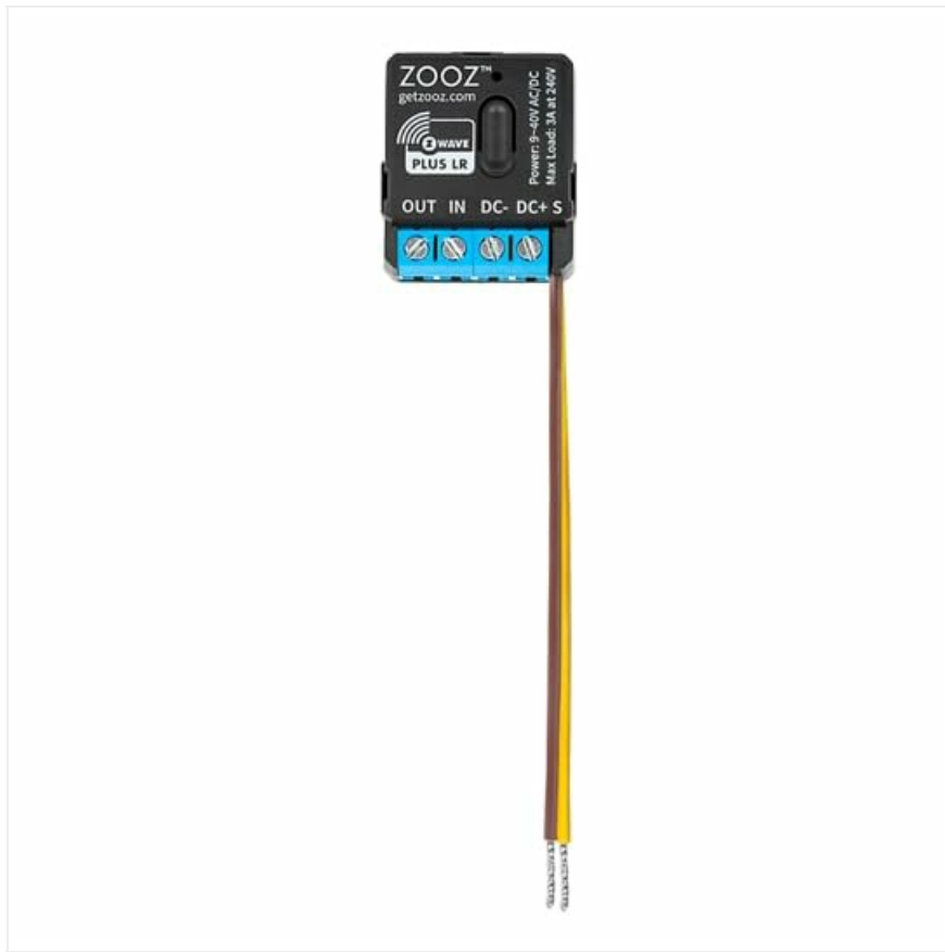
Front view of the ZEN58 800LR relay, illustrating the terminal block for power input (DC+, DC-), dry contact output (OUT), and dry contact analog input (IN, S).
