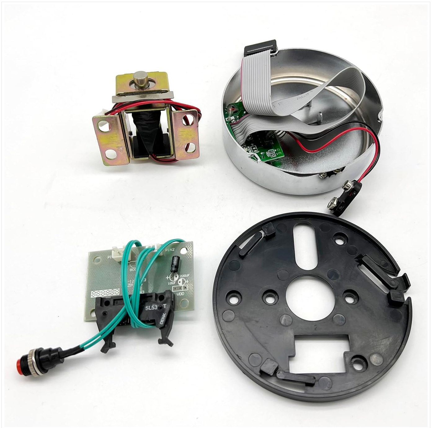
Image: Disassembled view of the lock, illustrating the internal components and where the battery connects.
