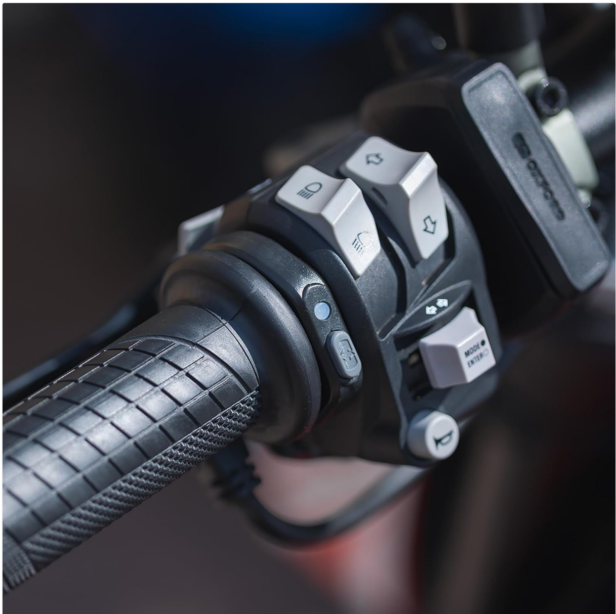
Figure 3: Integrated controller mounted on a handlebar.
