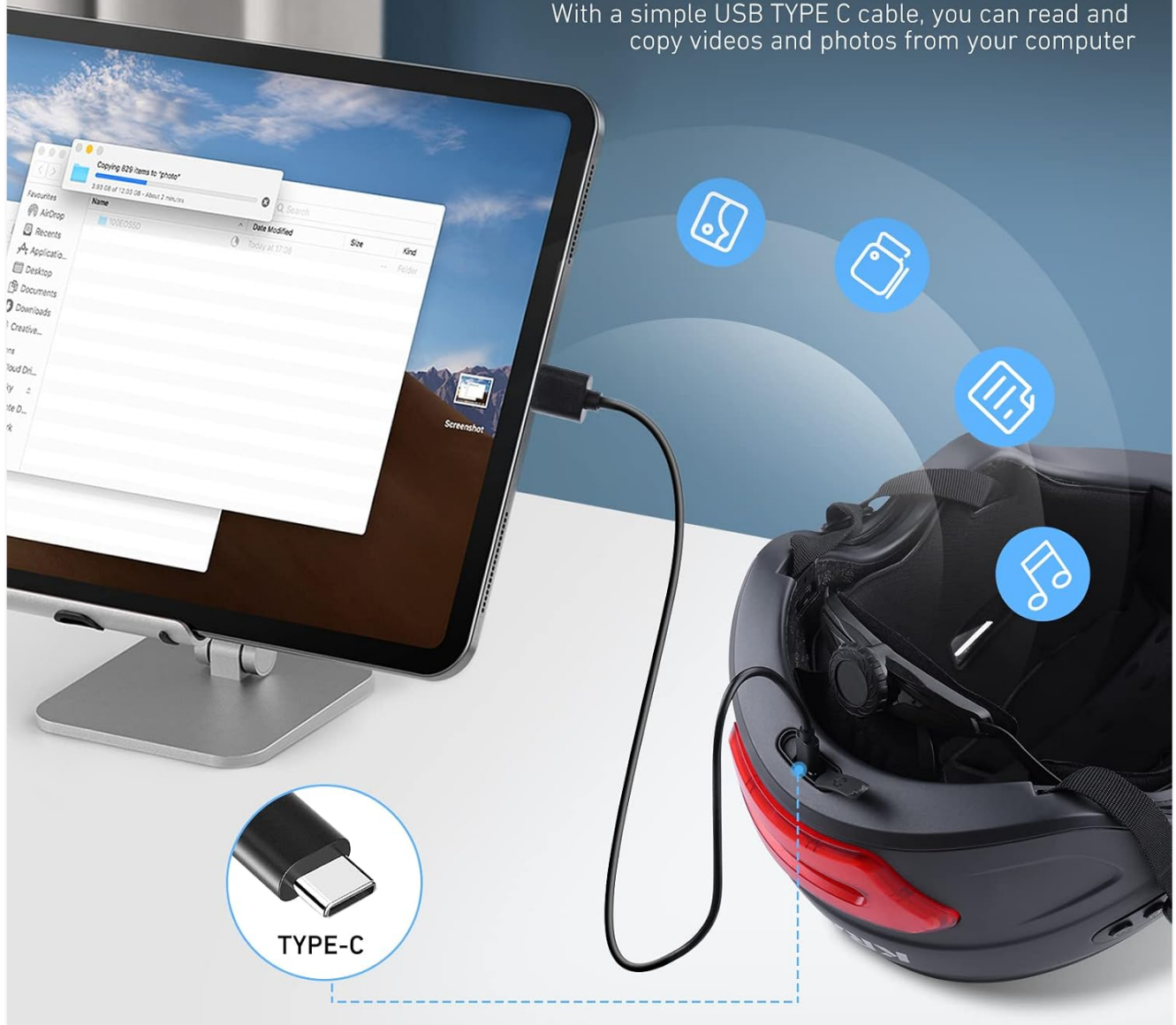
Figure 2: USB Type-C port for charging and data transfer.
