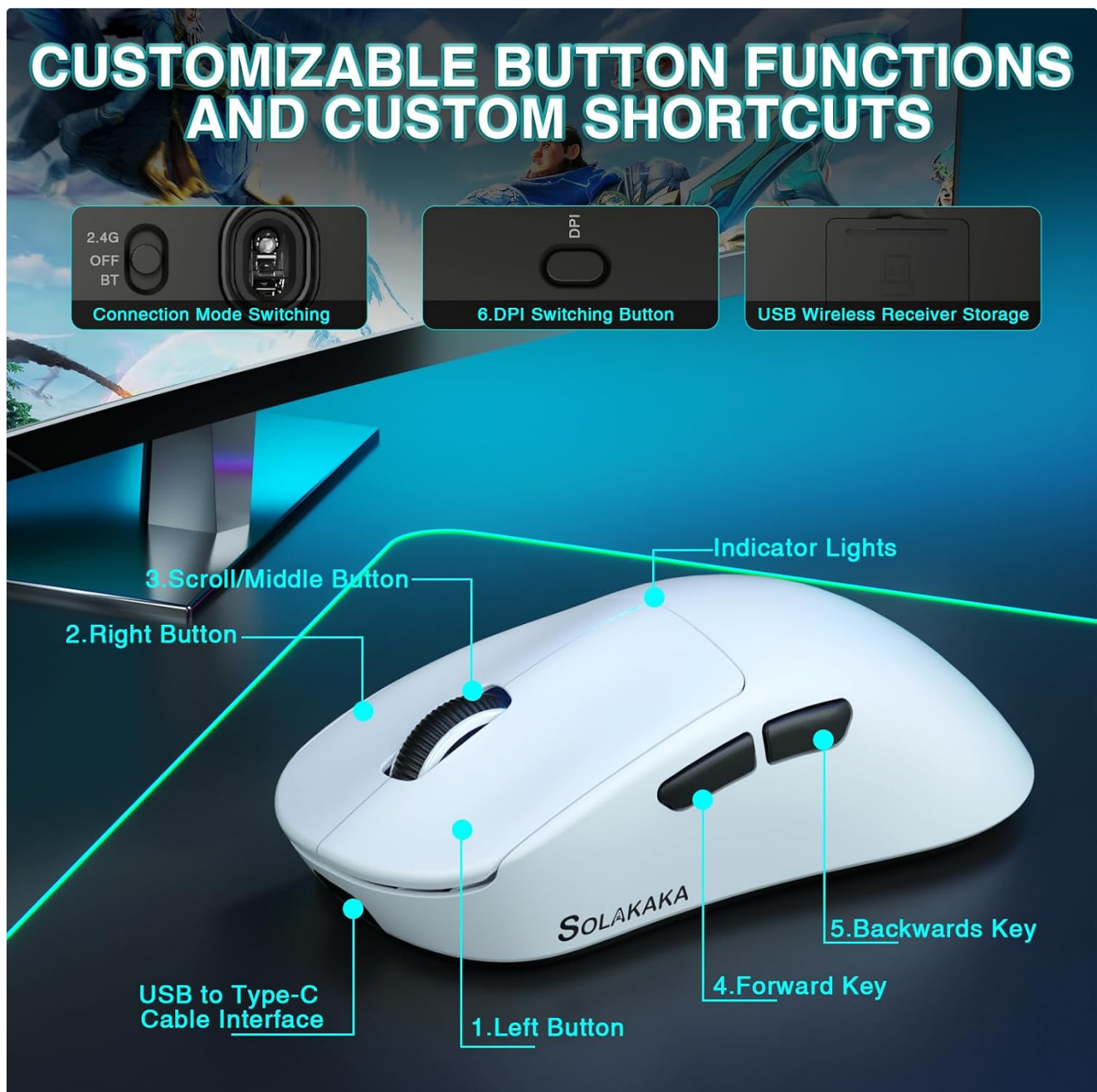
Image 4.5: Diagram illustrating the customizable button functions and layout of the SM850 mouse.
