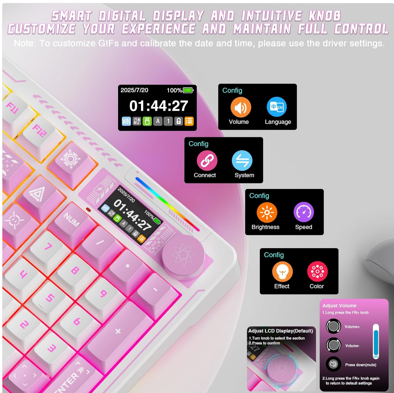
Image 2.1: Close-up of the LINGBAO K98 Pro's smart digital display and multi-functional knob.
