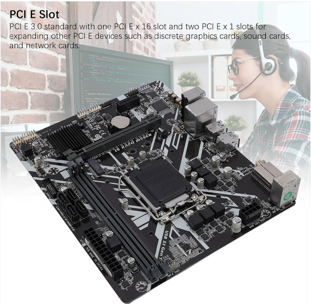
Figure 2.2: PCI E Slots. This image shows the PCI E 3.0 standard slots, including one PCI E x16 graphics slot and two PCI E x1 slots, allowing for expansion with discrete graphics cards, sound cards, and network cards.
