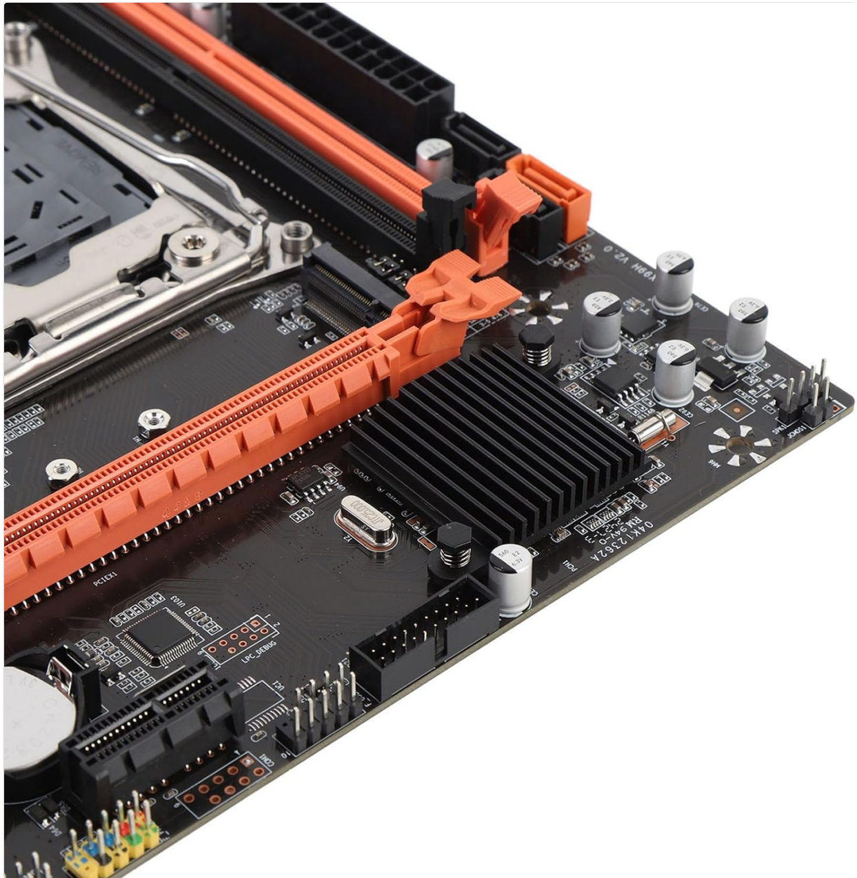
Figure 4.2: Close-up view of the M.2 slot and SATA ports.
