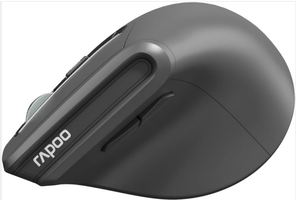
Image: Side view of the Rapoo EV310M Wireless Vertical Mouse, showing the forward and backward navigation buttons.
