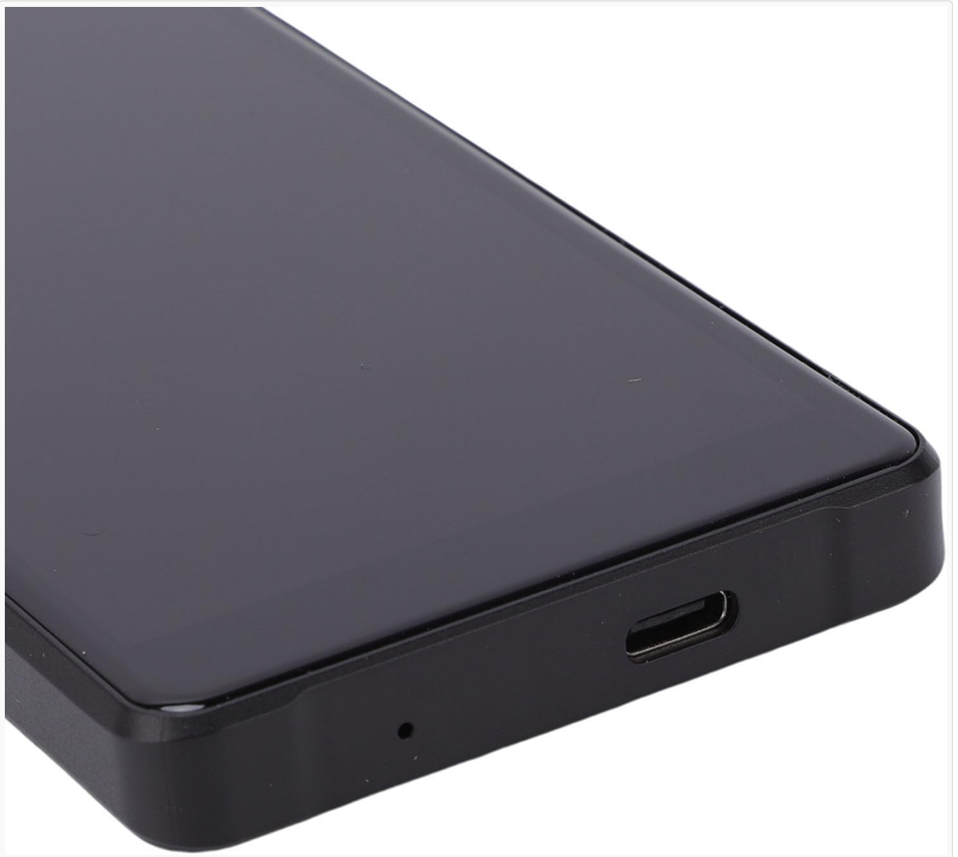
Figure 2: Charging Port. A close-up view of the bottom edge of the MP3 player, showing the USB Type-C charging port. This port is used for charging the device and for data transfer.
