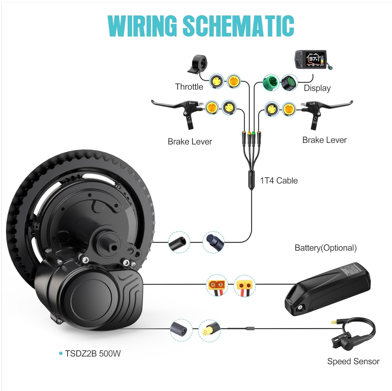
Image: Overview of the Varstrom mid-drive ebike conversion kit components, including the motor, chainring, and various cables.
