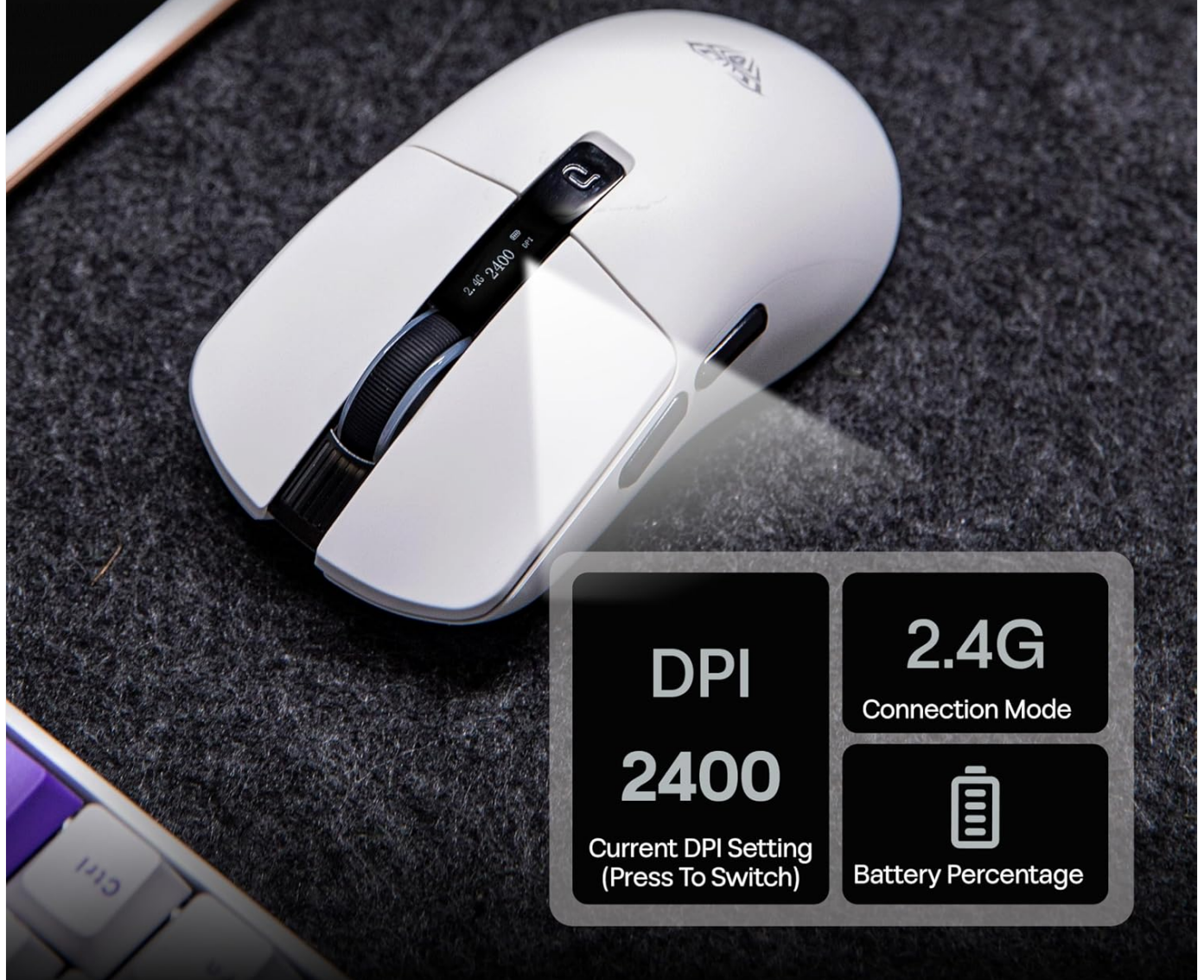
Figure 8: Display screen showing DPI and connection status.
