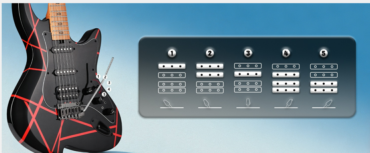
Figure 7: 5-Way Pickup Selector. This diagram shows the five different positions of the pickup selector switch and the corresponding active pickup configurations (e.g., bridge humbucker, bridge+middle, middle, middle+neck, neck single coil).
