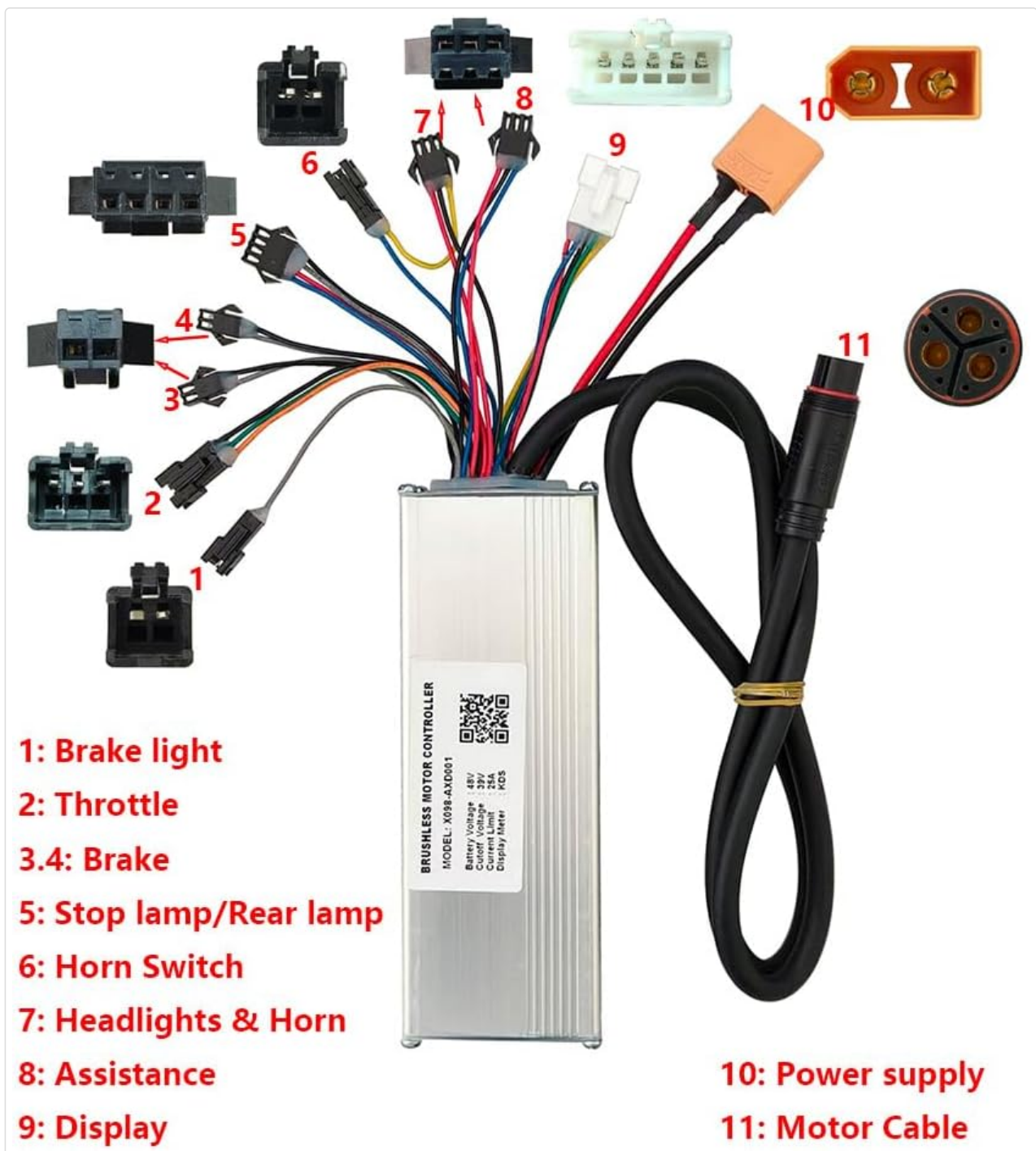
Figure 3: Wiring diagram illustrating the various interfaces of the X098-AXD001 Brushless Motor Controller.
