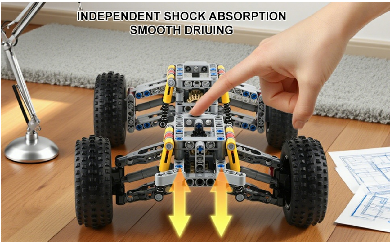
Figure 3.2: Demonstrating the independent shock absorption for smooth driving.
