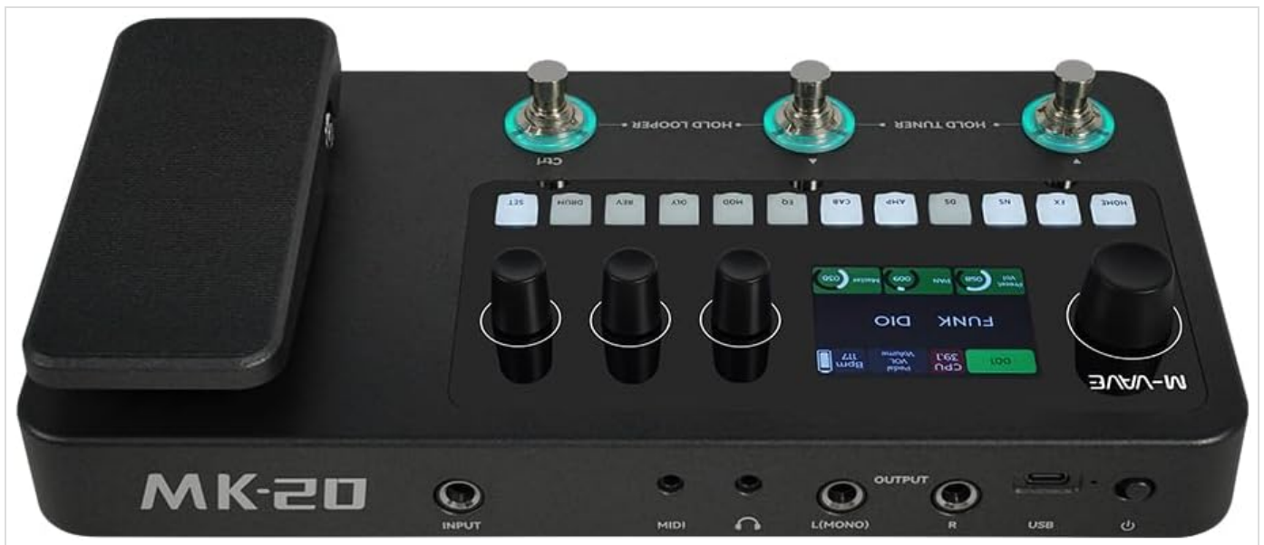
Figure 4.3: Rear view of the M-VAVE MK-20 Multi-Effect Processor, displaying the input/output jacks, MIDI port, headphone jack, USB-C port, and power button. This image details all available connectivity options.
