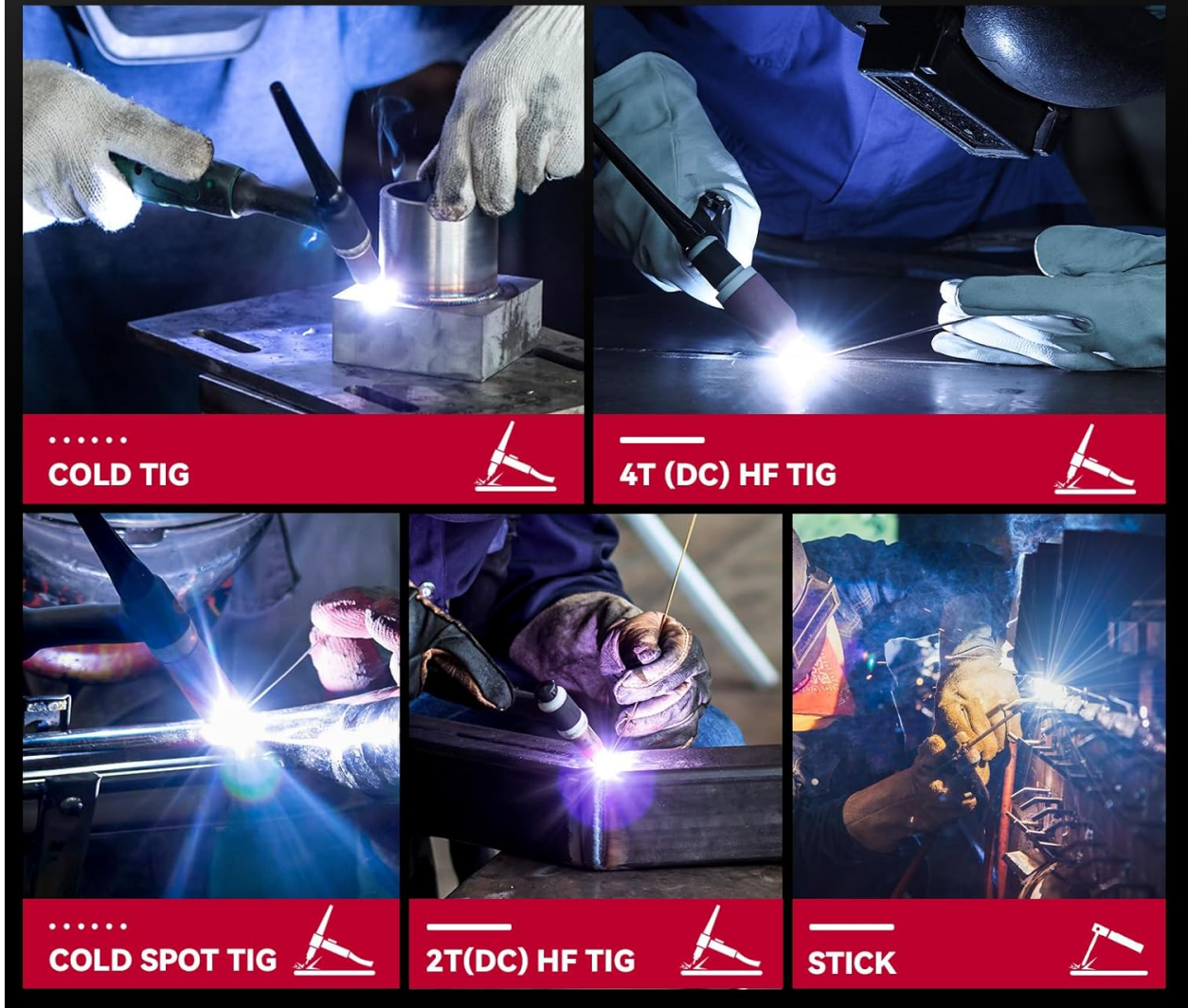
Figure 3: Visual representation of the five welding modes: Cold TIG, 4T (DC) HF TIG, Cold Spot TIG, 2T (DC) HF TIG, and Stick welding, demonstrating the versatility of the machine.
