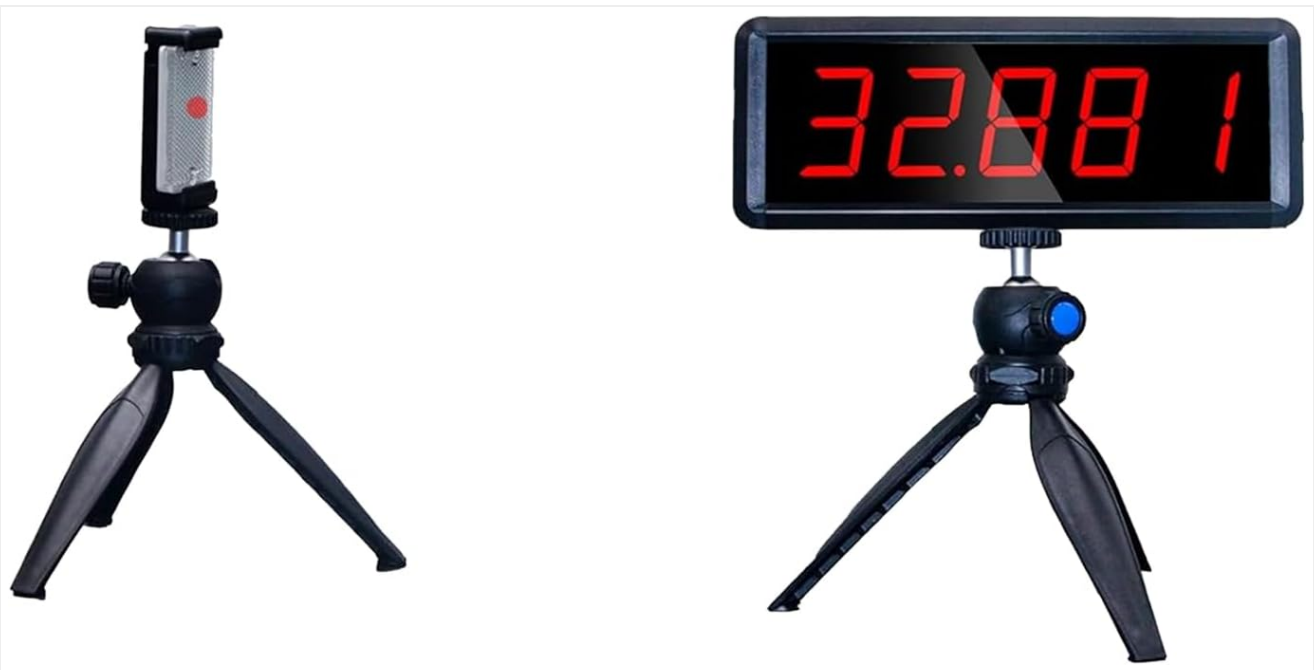
Image 1.1: The Ousmile Wireless Laser Timer (right) and its reflector (left), each mounted on a tripod.
