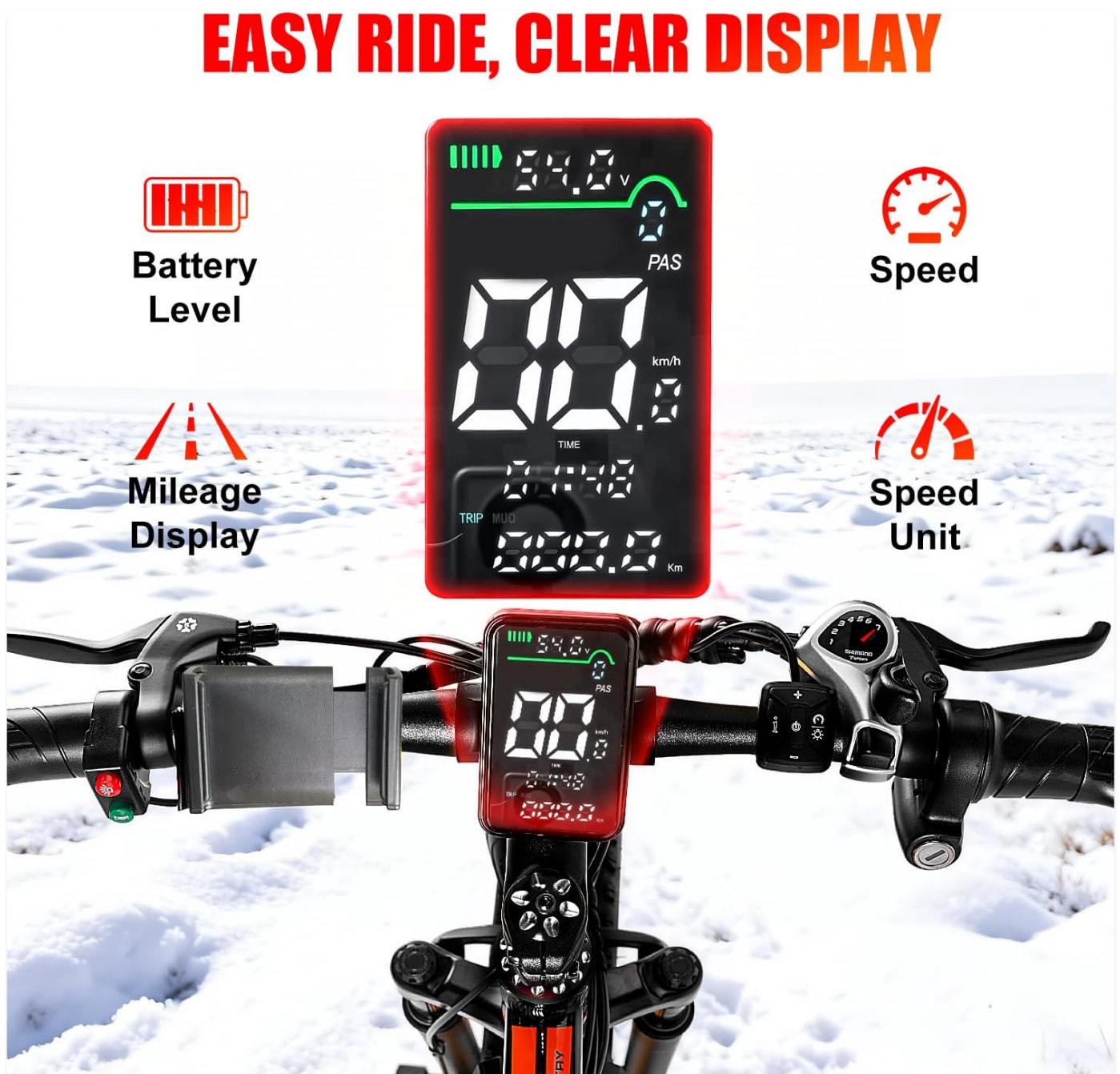
Image: The clear LED display of the EOEOTWO E01 Electric Bike, showing battery level, speed, mileage, and speed unit.
