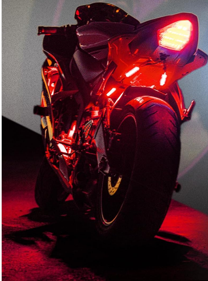
Figure 3.1: Motorcycle displaying red underglow lights when the brake is applied, enhancing safety.
