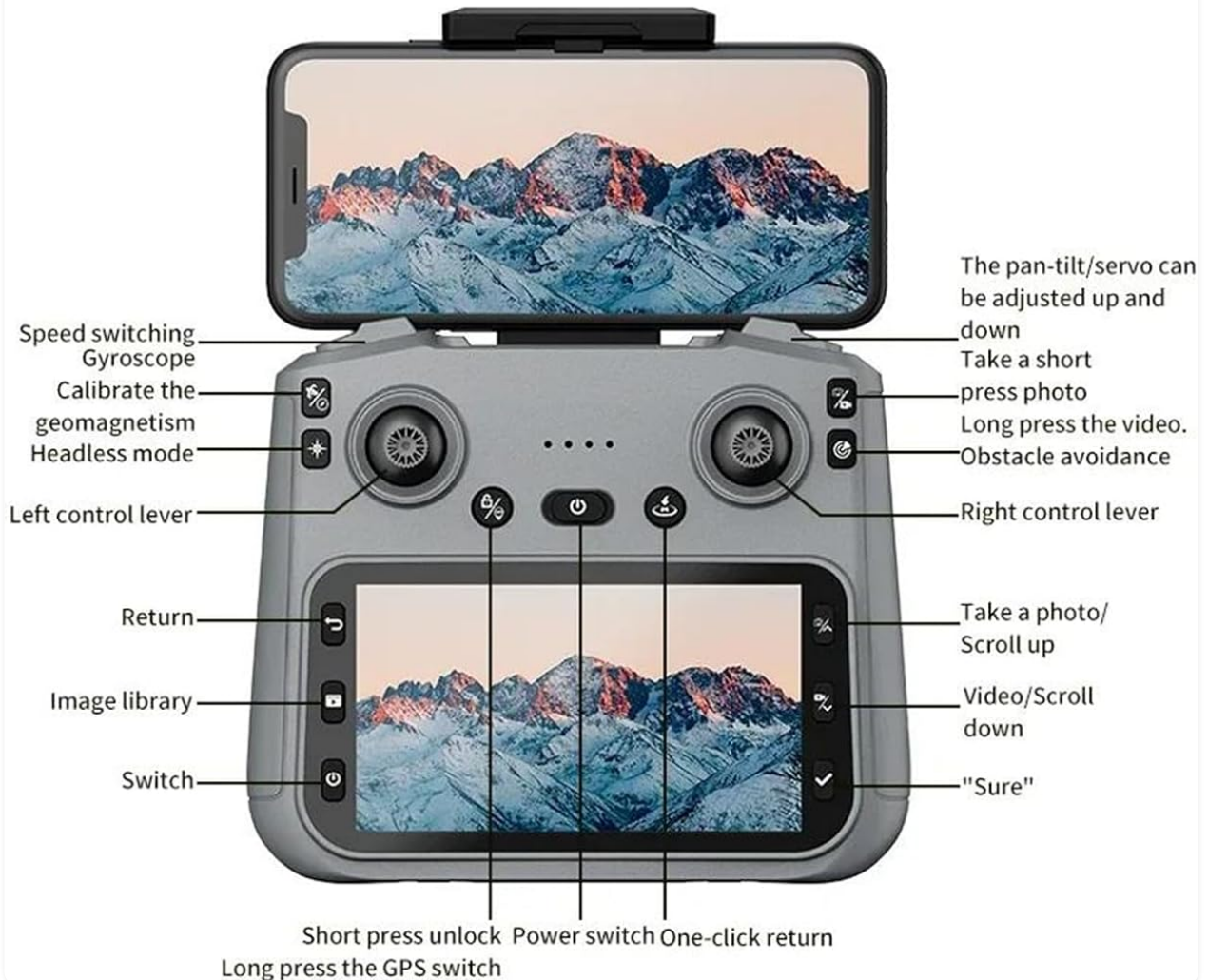
Figure 2.3: Remote Control Guide. Key controls include: Speed switching, Gyroscope, Calibrate geomagnetism, Headless mode, Left control lever, Return, Image library, Switch, Short press unlock, Power switch, One-click return, Long press GPS switch, Pan-tilt/servo adjustment, Take a short press photo, Long press video, Obstacle avoidance, Right control lever, Take a photo/Scroll up, Video/Scroll down, and 'Sure' button.
