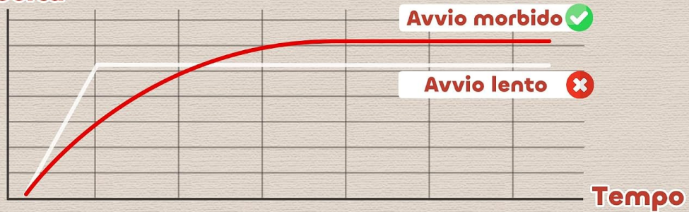
Image 4.2: Soft-start technology for smooth acceleration.
