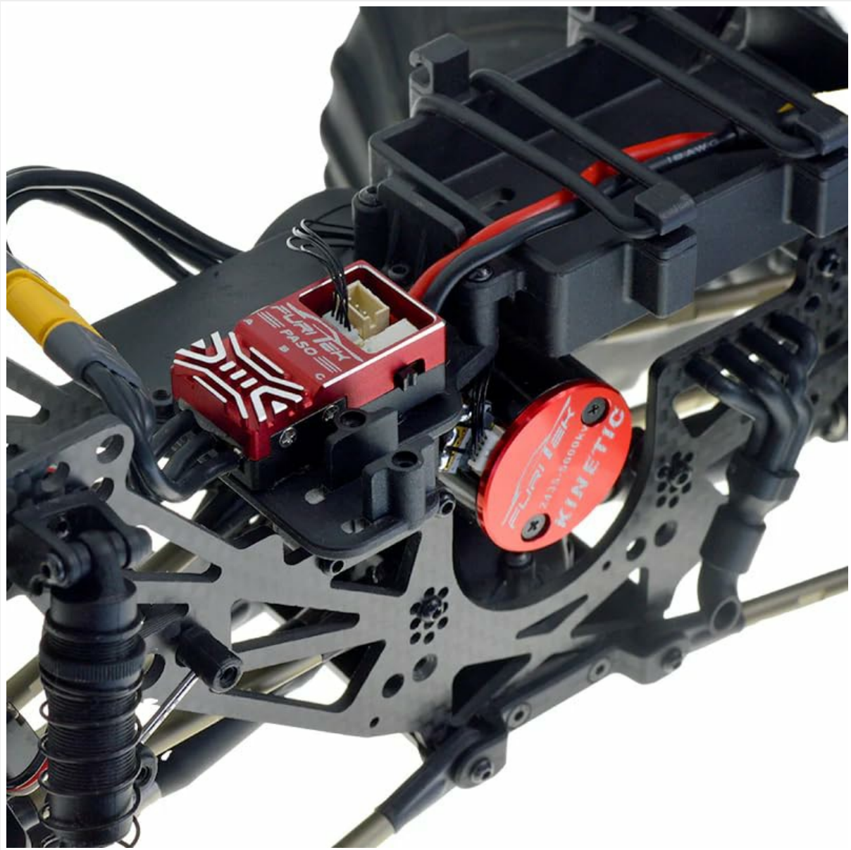
Image: A close-up view of the Furitek Predator ESC and Kinetic motor installed within an RC vehicle chassis.
