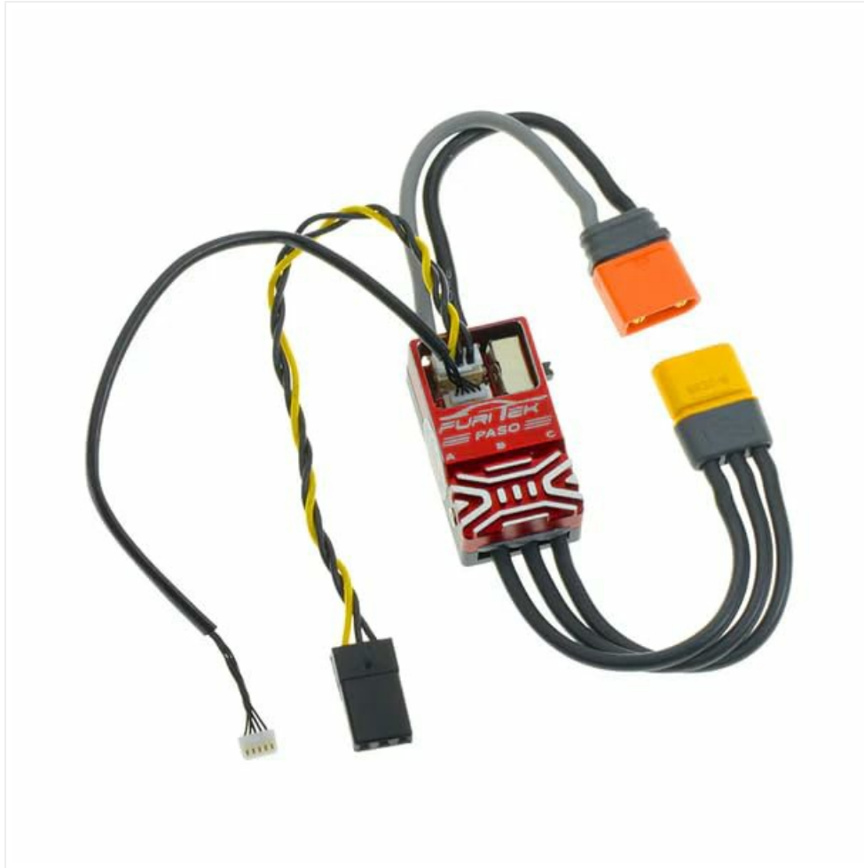
Image: The Furitek Predator ESC showing connected motor wires, sensed cable, and battery connector.
