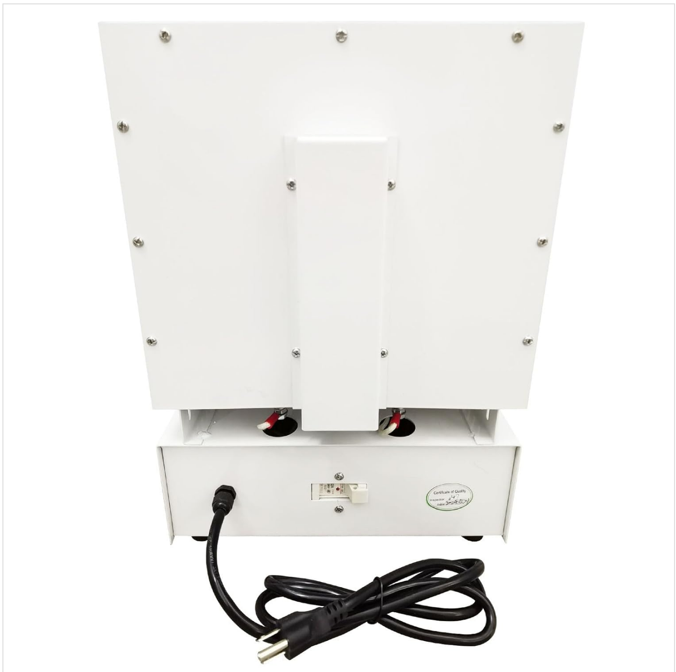
Figure 4.1: Rear view of the furnace, illustrating the power connection point.
