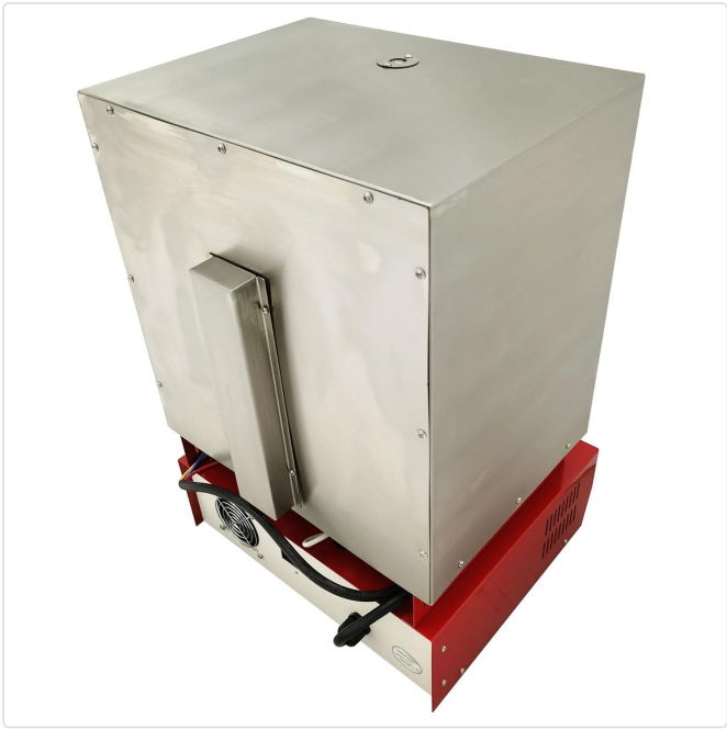
Figure 2.8: Rear View. The rear view of the furnace, illustrating the power input connection and additional ventilation grilles for heat dissipation.
